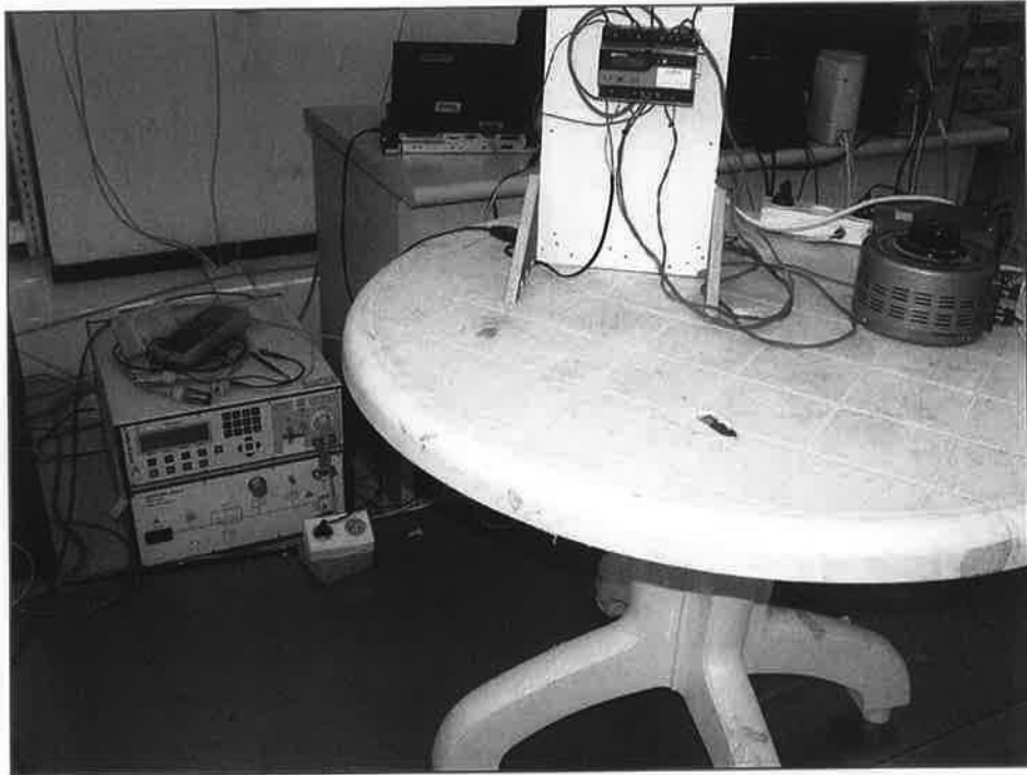
Photograph: 7.2: EFT test on 3 phase AC
