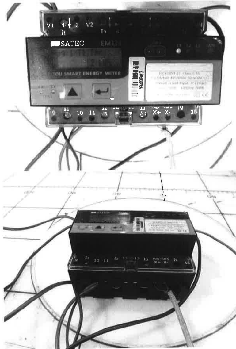
Picture #5 EM133 Radiated emission test setup
