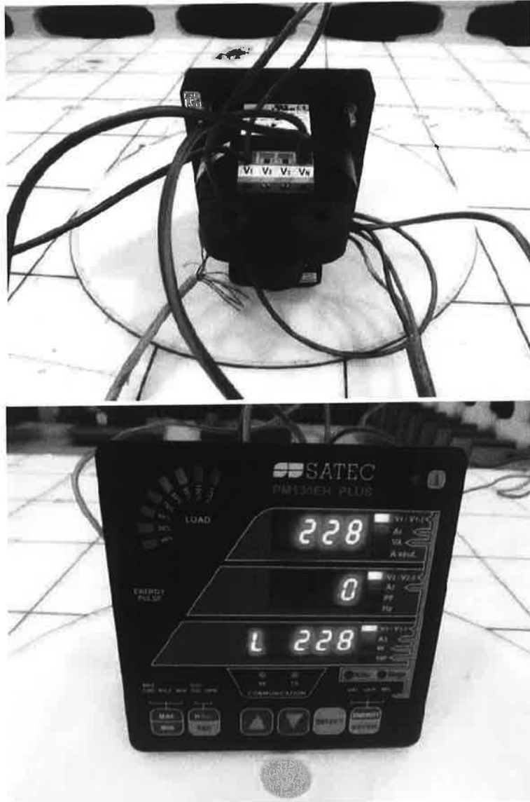
Picture #2 PM 130 Plus Radiated emission test setup
