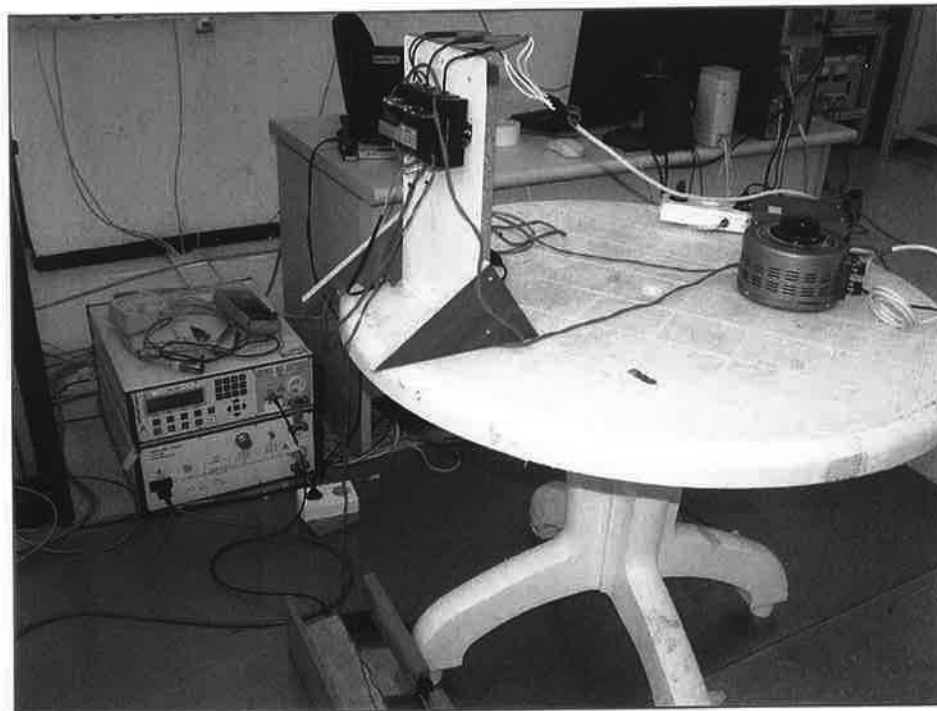
Photograph 7.3: EFT test on RS 485
