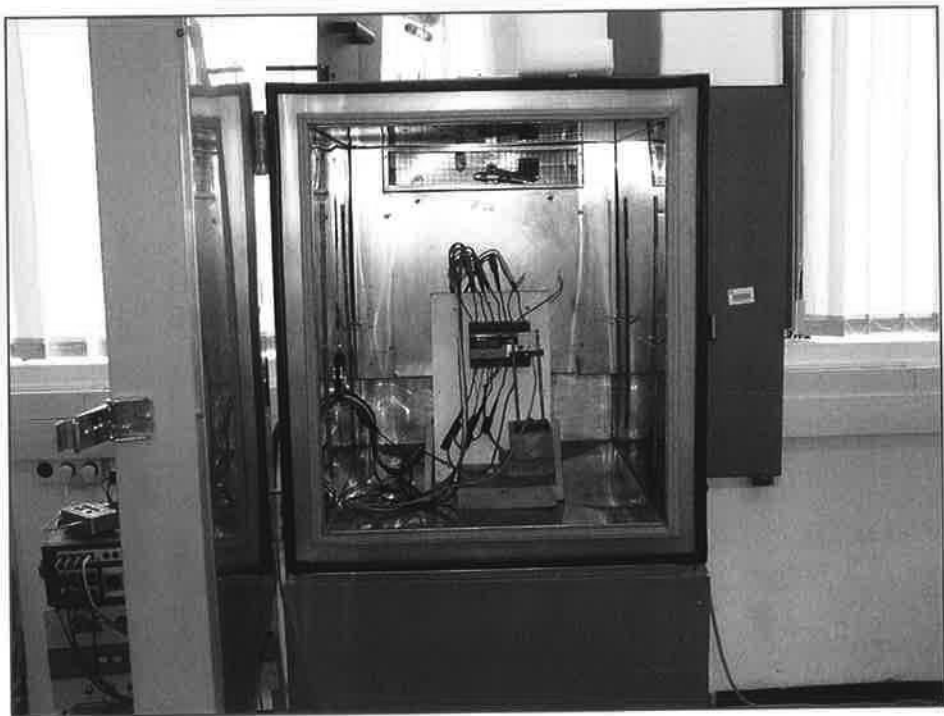
Photograph 12: Variations due to ambient temperature Test
